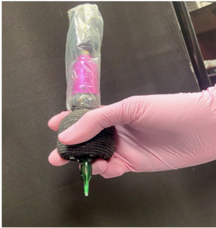
Figure 2. Rotary pen-style tattoo machine wrapped for hygiene; its lightweight body and minimal vibration make it a popular choice for fine lines [13]
