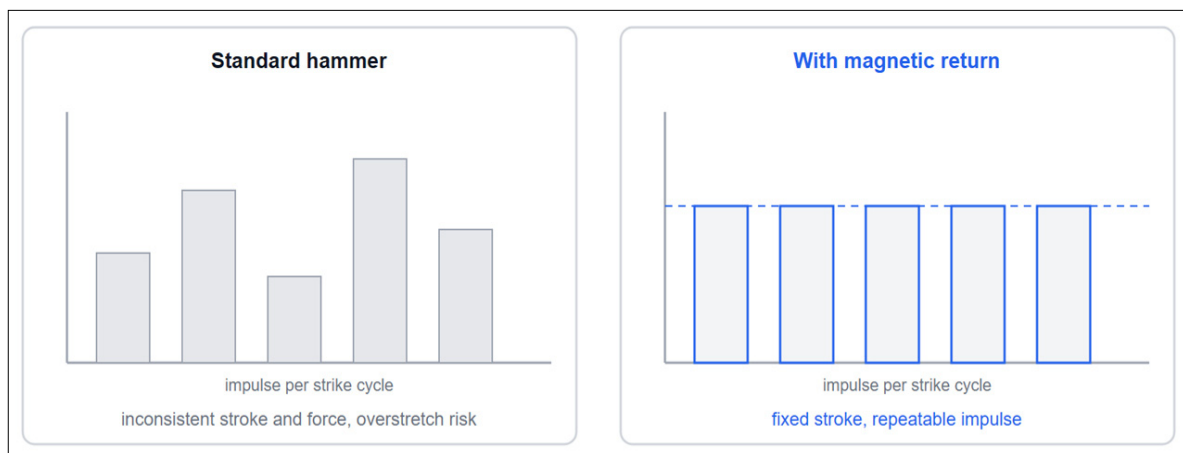
Fig. 2. Strike-cycle comparison: standard hammer and magnetic-return hammer.
